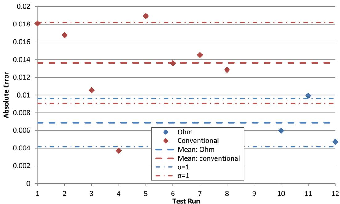
**Figure 6-1** Comparison of errors for all test runs on both Ohm and conventional meter with standard deviation of  $\sigma=1$
