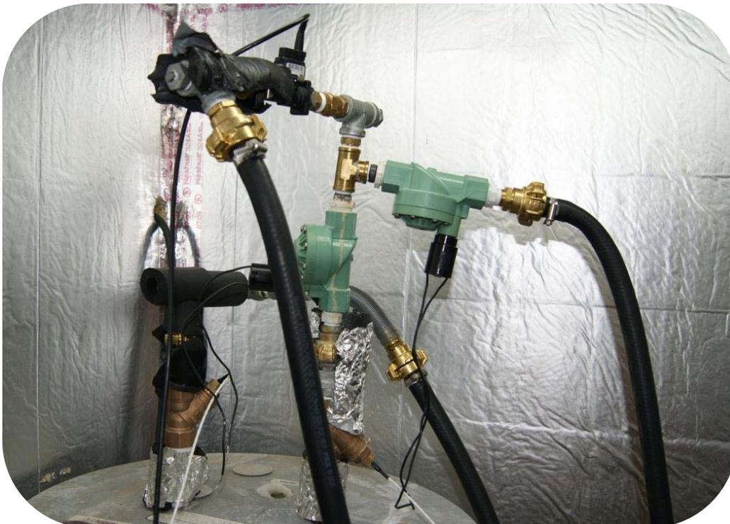
Figure 3-3 Photo of test setup for evaluation Sunnovations, Inc. Ohm heat meter
