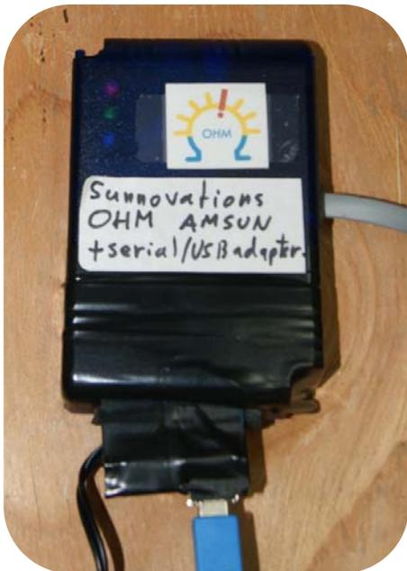
**Figure 3-1** Photo of Sunnovations, Inc. **Ohm** Heat Meter computer with modification for serial communication output
